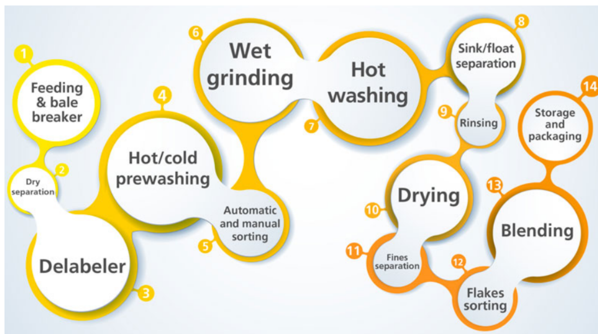
Figure 29: PET Bottles to Flakes Process (Sorema, 2023)
